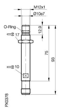
**Inductive Sensors** BES 516-300-S 163-S 4-D M12x1 x 93 normally-open Sn=1,5mm shielded pressure rated to 500 bar
